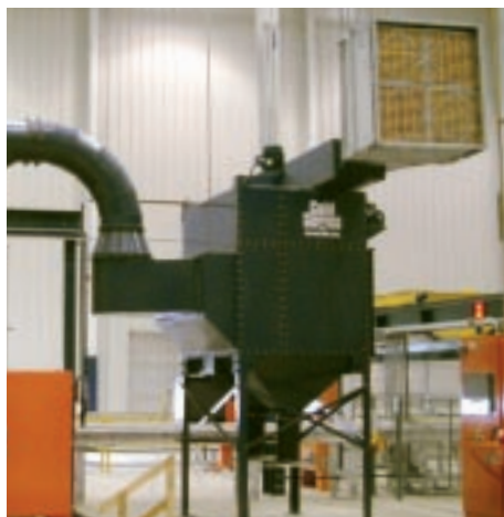
Abrasive Resistant Inlet, Top Mount Fan, Silencer, & Safety Monitoring Filter
