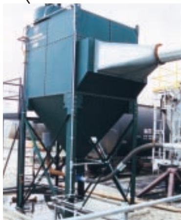
High Entry Inlet Cross flow is created through the filters. Eliminates upward "can" velocities associated with traditional hopper inlets.
