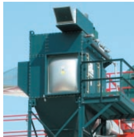
Explosion Vent—NFPA Rupture Panel
