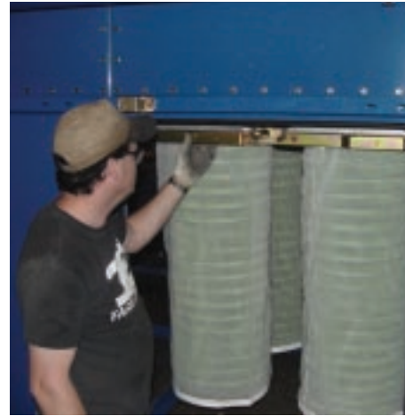
Overbag Option for Fibrous Dusts like Paper & Fiberglass
